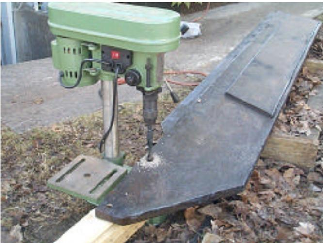
**39. Drilling out the pivot hole for a larger size bolt**
