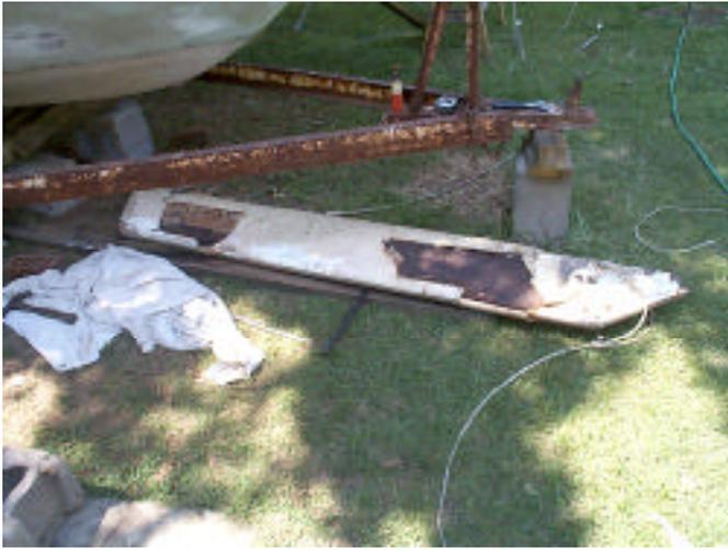
**36. The keel removed, the boat back down on the trailer.**
