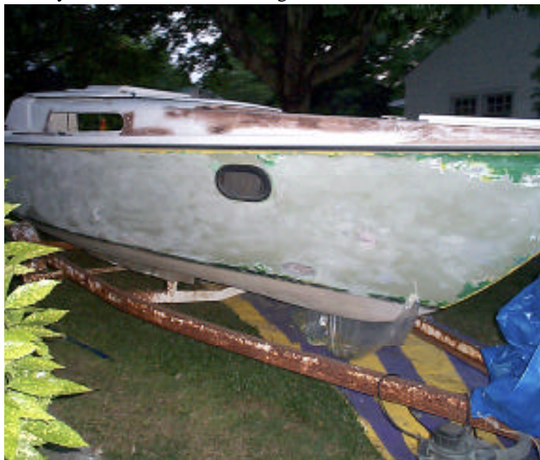
69. The exterior paint job at the start of the project. A little more scraping and sanding remains to be done around the bow.
