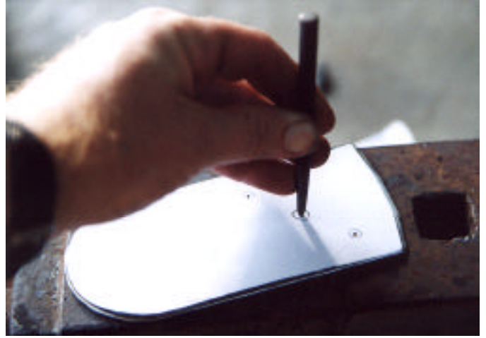
98. Centerpunch the holes for drilling
