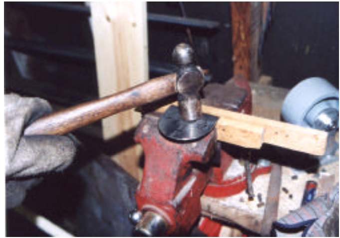
102. Bend the bracket at the marks using a bench vise. Using wood blocks prevents scratches.
