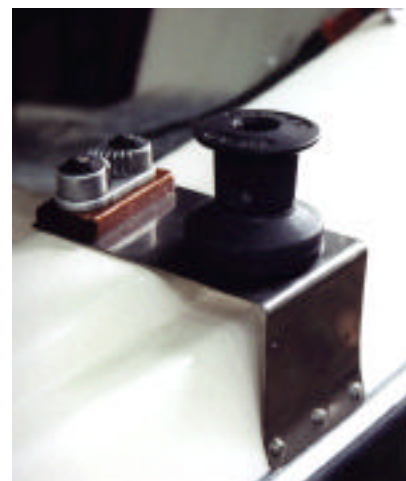
104. I built these winch bases using identical methods as the bow light bracket.
