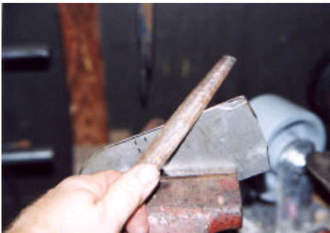
99. Round sharp edges with a file and/or sandpaper
