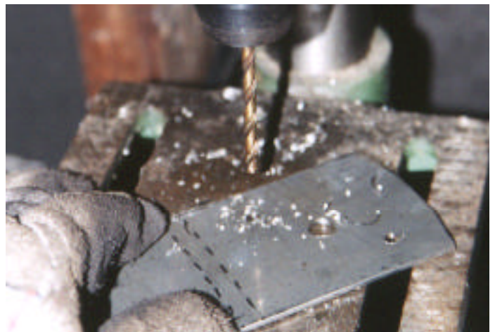
100. Drill the holes using a drill press and cobalt bits.
