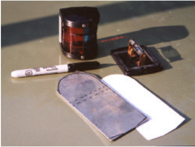
97. A stainless bracket for the bow light. Start with a paper pattern, mark the bends and mounting holes.
