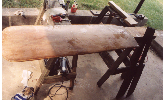
a80. The lower rudder saturated easily, and now is ready for sanding and painting.
